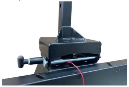
2. Apply provided lock tight to the threads of the plunger pin. Thread plunger pin into truck side hinge, making sure everything functions properly, tighten plunger pin and hinge pin.
